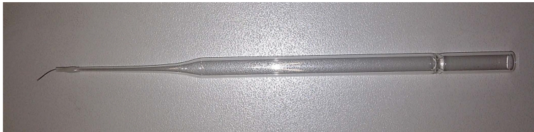
Figure 5. Preparing a hairpin pick for gentle manipulation of C. elegans . Remove a hair from your eyebrow and glue it to the tip of a glass Pasteur pipette or a toothpick.
